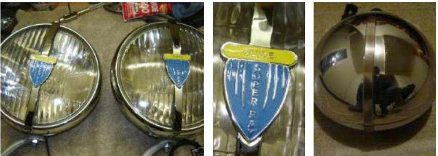
*The helmet at the top in the prior version has been removed and a decorative band has been added to the shell which extends to the back of the lamp.*
