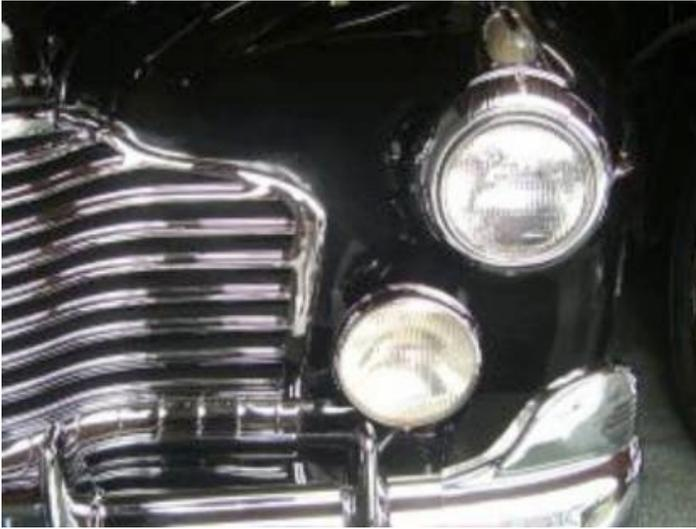
1941 Buick with 6-11/16" Light mounted as specified in Buick Service Bulletins.
