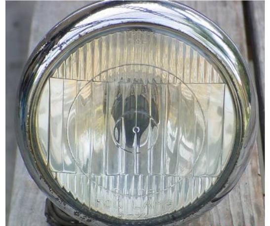
*The Guide round (Guide part number unknown) 5-3/4" light was designed for the 1941 Oldsmobile and has a unique circular pattern on the lens (this light is shown in 1941 Oldsmobile literature).*
