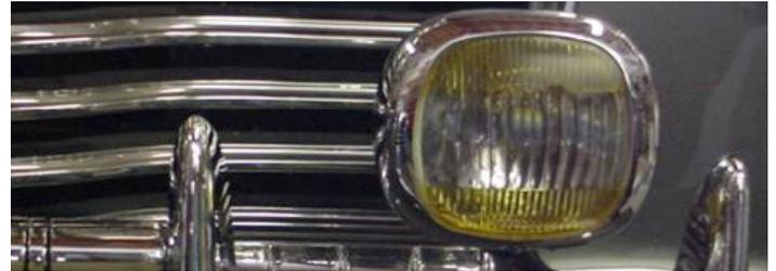
*Close-up view showing light mounting. Note position closer to center obtained by reversing the Guide mounting brackets from that specified in the Buick Service Bulletin.*
