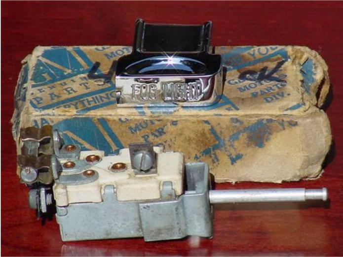
*This was a switch specifically intended for these lights and mounted on the right side of the center dash panel. The "ACCESSORY" labeled knob was removed and replaced with the "FOG LIGHT" knob when these lights were installed in 1941.*
