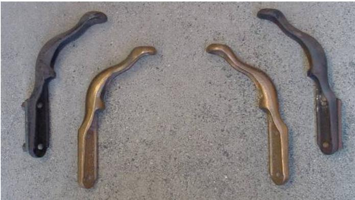
*The Buick part numbers for the brackets were 5932053 Left and 5932054 Right. The cast iron brackets were painted semi-gloss black. The clamps were cadmium plated.*
